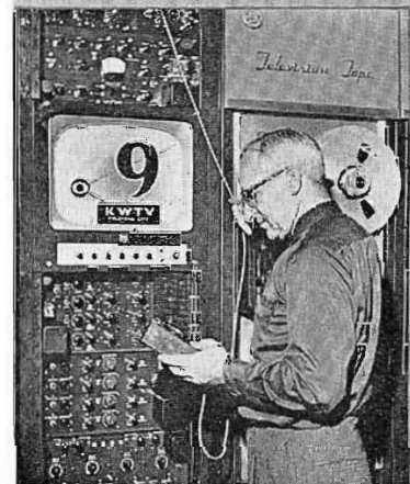
Electronic quadrature adjustment, an exclusive RCA feature, assures the best picture accuracy in seconds, even in playing back tapes made on other recorders. Here, Maintenance Engineer Charlie Sheaffer checks voltage output before a taping session.
