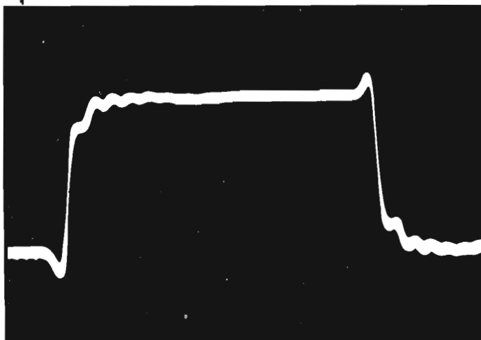
FIG. 1. Typical uncorrected TV system response of 100 kc square wave.
