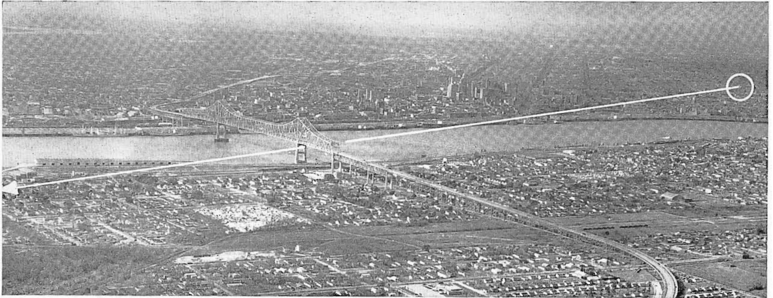
FIG. 12. Path of microwave transmission at WWL-TV runs from studio at upper right, under Mississippi River bridge, to transmitter (beyond picture at extreme left).
