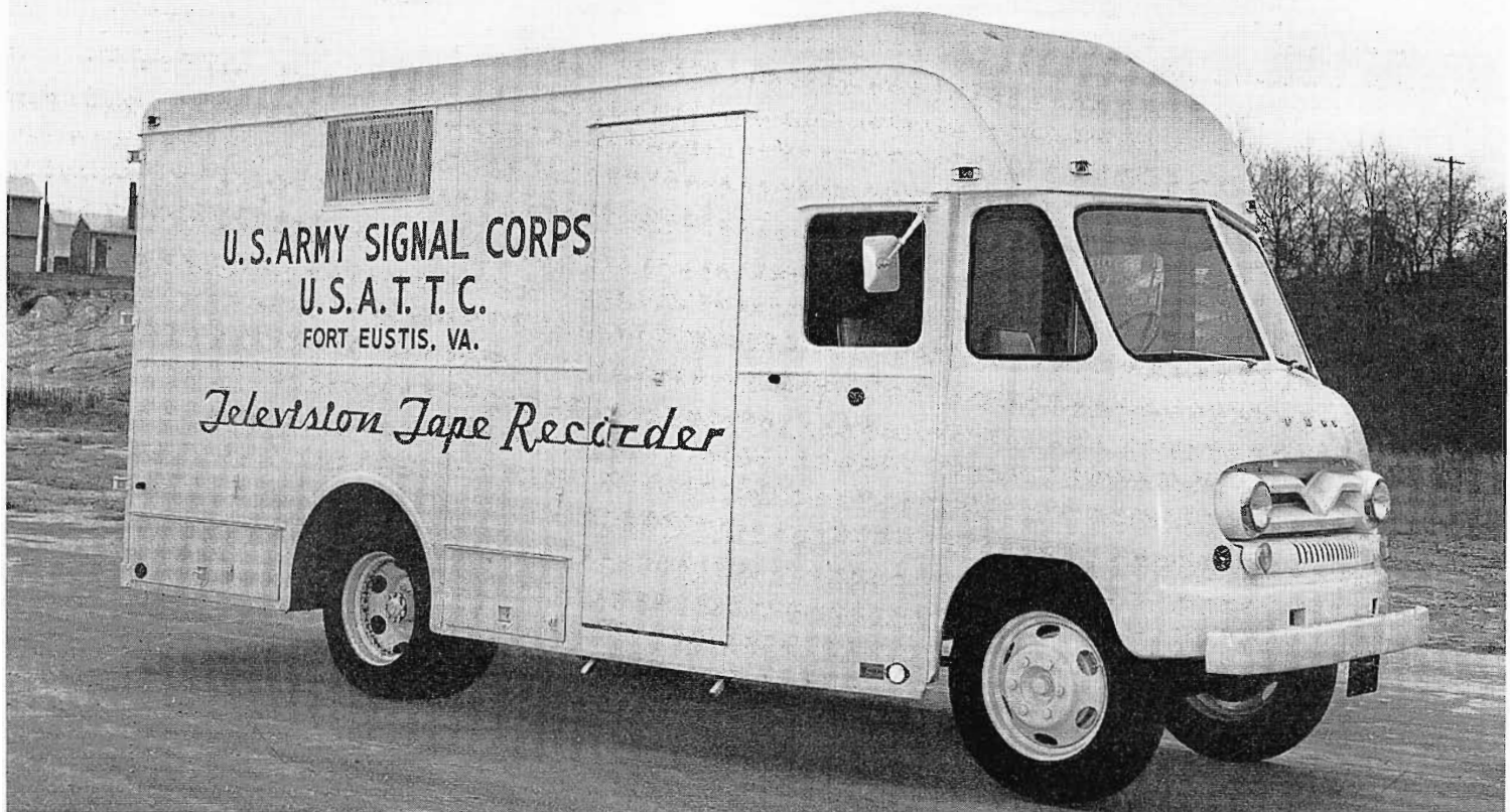
FIG. 1. Army Transportation School uses this TV Tape Mobile unit for spot pickups at widely separated points on the Ft. Eustis base. These pickups are then incorporated into the training program via closed circuit television.
